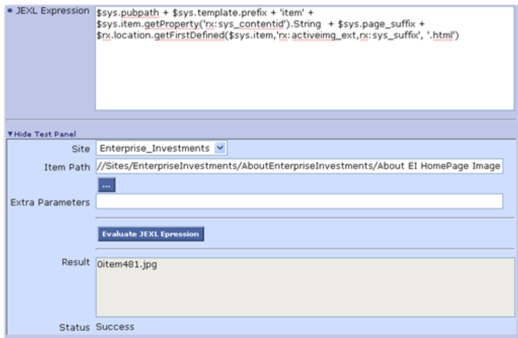
Figure 244: Testing a JEXL showing a Status of success while producing an erroneous output
