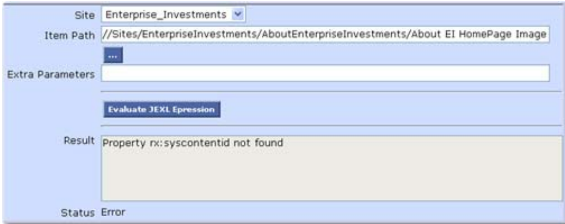
Figure 243: Test Panel showing an error in the JEXL expression. In this case the property rx:sys_contentid was specified incorrectly without an underscore.
